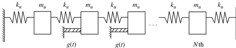
Figure 1. Linear array of  $N$  spring-mass oscillators used for numerical studies,  $N = 30$ ,  $m_u = 1$  kg,  $k_u = 4 \times 10^5$  N/m.
